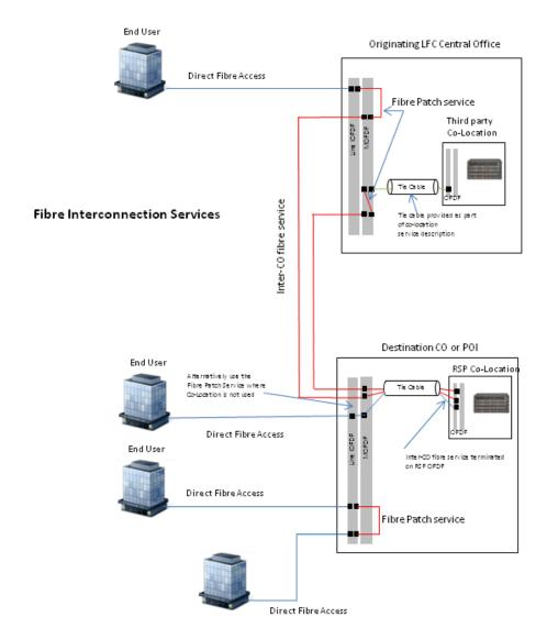
This is a generic diagram showing the standard configuration of the Fibre Patching Service, and the Inter-CO Fibre Service with and without an RSP Co Location footprint. It is not intended to represent every situation.
